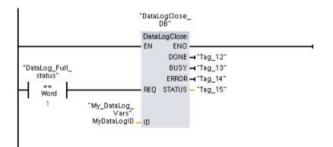
**Network 7** A positive signal edge DataLogOpen REQ input simulates the user pushing a button on an HMI that opens a data log file. If you open a Data log file that has all records filled with process data, then the next DataLogWrite operation will overwrite the oldest record. You may want to preserve the old Data log and instead create a new data log, as shown in network 7.
