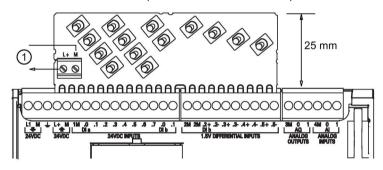
① 24 VDC sensor power out
