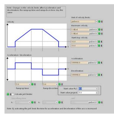
The figure above shows the Motion parameter screen with compare icons showing which values are different between online and offline projects. A green icon indicates that the values are the same; a blue/orange icon indicates that the values are different.
