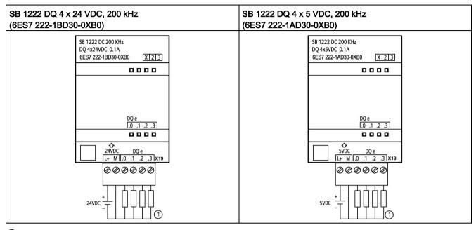
Table A- 188 Wiring diagrams for the 200 kHz digital output SBs
