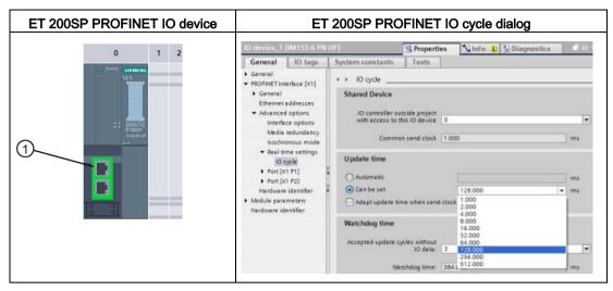
Table 11-54 Configuring the ET 200SP PROFINET IO cycle time
