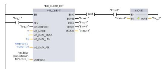
**Network 2:** Modbus function 2 - Read 32 input bits from a Modbus TCP server with the IP address assigned in "Modbus connections".TCPactive\_1.
