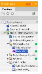
When you have connected to the CPU, STEP 7 turns the headers of the work areas orange.
