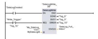
**Network 6** Close the data log once the last record has been written. After executing the DataLogWrite operation that writes the last record, the log file full status is signaled when DataLogWrite STATUS output = 1.
