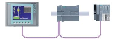
If a CM 1242-5 and a CM 1243-5 are installed together, an S7-1200 can perform as both a slave of a higher-level DP master system and a master of a lower-level DP slave system, simultaneously:
