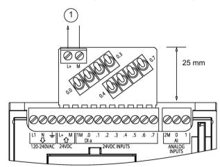
① 24 VDC sensor power out
