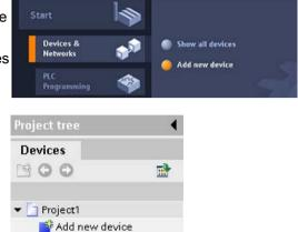
Be sure you insert the correct model and firmware version from the list. Selecting the CPU from the "Add new device" dialog creates the rack and CPU.
