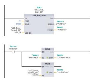
Network 1"PortStatus"port status and"USS\_Drive\_Control\_DB".USS\_Ex tended\_Error extended error code values are only valid for one program scan. The values must be captured for later processing. Network 2The "PortError" contact triggers the storage of the "PortStatus" value in "LastPortStatus" and the"USS\_Drive\_Control\_DB".USS\_Ext ended\_Error value in "LastExtError".
