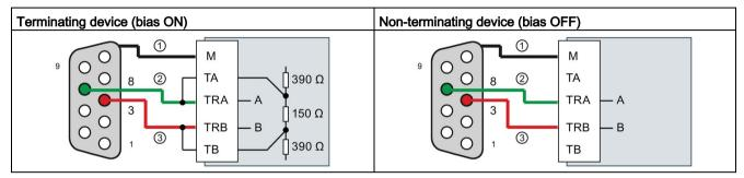
① Connect M to the cable shield
