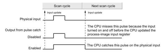
Because the pulse catch function operates on the input after it passes through the input filter, you must adjust the input filter time so that the pulse is not removed by the filter. The figure below shows a block diagram of the digital input circuit:
