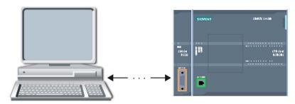
You must connect the communication interface of the CM 1241 RS232 module to the RS232 interface of the PC, which is normally COM1. Because both of these ports are Data Terminal Equipment (DTE), you must switch the receive and transmit pins (2 and 3) when connecting the two ports, which you can accomplish by either of the following methods:
