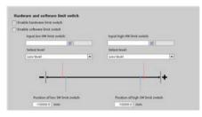
Configure the properties for the drive signals, drive mechanics, and position monitoring (hardware and software limit switches).
