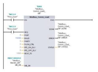
One Modbus\_Master instruction is used in the program cycle OB to communicate with a single slave. Additional Modbus\_Master instructions can be used in the program cycle OB to communicate with other slaves, or one Modbus\_Master FB could be re-used to communicate with additional slaves.
