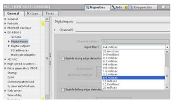
Each input point has a single filter configuration that applies to all uses: process inputs, interrupts, pulse catch, and HSC inputs. To configure input filter times, select "Digital Inputs".
