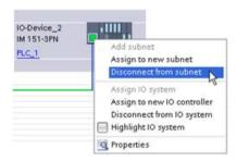
Right-click the interface port of the network device and select the "Disconnect from subnet" command from the context menu.
