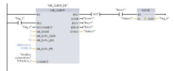
Network 1: Modbus function 15 - Write output bits in a Modbus server
