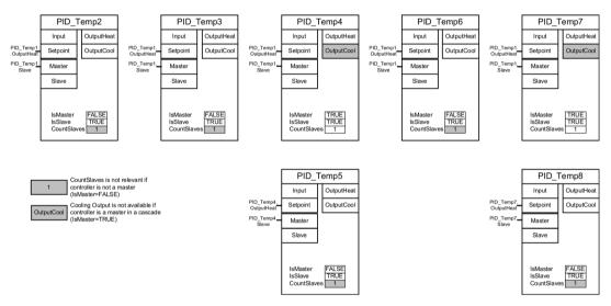
Figure 10-8 PID\_Temp\_Cascading\_communication\_connection
