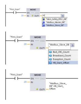
Entering a Modbus slave variable using the default DB name:
