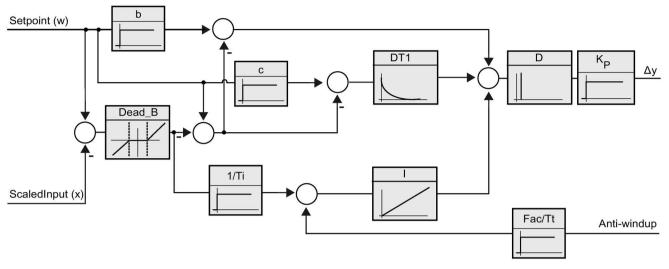
Figure 10-3 Operation of the PID\_3Step controller as a PID T1 controller with anti-windup
