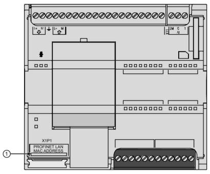
The MAC address is printed on the front, lower-left corner of the CPU. Note that you have to lift the lower door to see the MAC address information.
