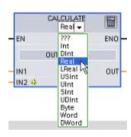
Click the "???" and select the data types for the input and output parameters. (The input and output parameters must all be the same data type.)
