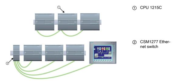
The CPU 1215C and the CPU 1217C have a built-in 2-port Ethernet switch. You can have a network with a CPU 1215C and two other S7-1200 CPUs. You can also use the rack-mounted CSM1277 4-port Ethernet switch for connecting multiple CPUs and HMI devices.
