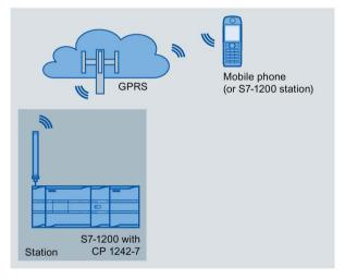
A SIMATIC S7-1200 with a CP 1242-7 can send messages by SMS to a mobile phone or a configured S7-1200 station.
