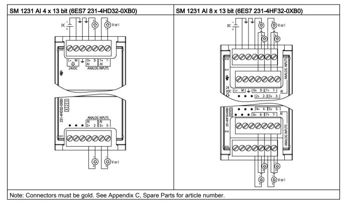
Table A- 136 Wiring diagrams for the analog input SMs
