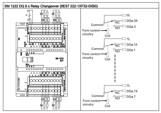
A changeover relay output controls two circuits using a common terminal: one normally closed contact, and one normally open contact. Using output "0" as an example, when the output point is OFF, the common (0L) is connected to the normally closed contact (.0X) and disconnected from the normally open contact (.0). When the output point is ON, the common (0L) is disconnected from the normally closed contact (.0X) and connected to the normally open contact (.0).
