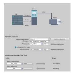
After you create the technology object for the axis, you configure the axis by defining the basic parameters, such as the PTO and the configuration of the drive interface. You also configure the other properties of the axis, such as position limits, dynamics, and homing.
