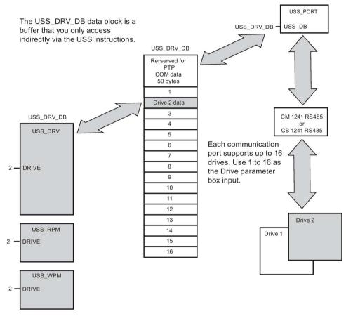
All drives (up to 16) connected to a single RS485 port are part of the same USS network. All drives connected to a different RS485 port are part of a different USS network. Each USS network is managed using a unique data block. All instructions associated with a single USS network must share this data block. This includes all USS\_DRV, USS\_PORT, USS\_RPM, and USS\_WPM instructions used to control all drives on a single USS network.
