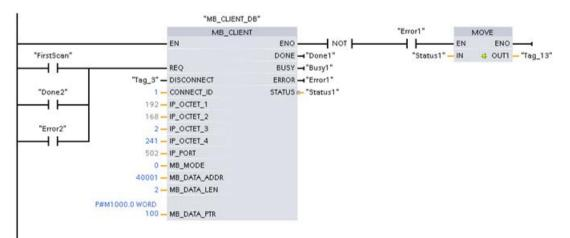
Network 1: Modbus function 3 - Read holding register words
