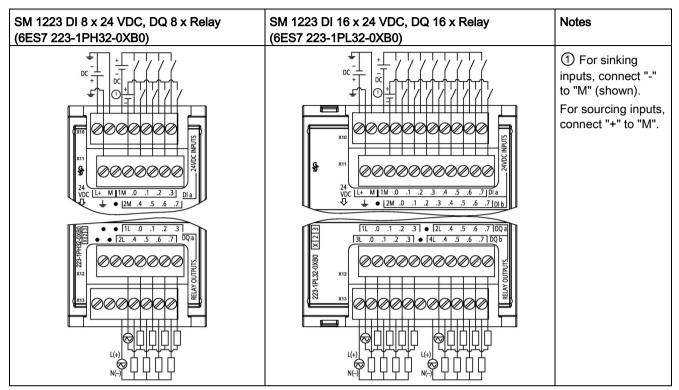
Table A- 122 Wiring diagrams for the digital input VDC/output relay SMs
