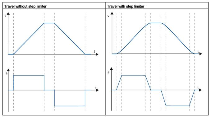
The jerk limit gives a "smoothed" velocity profile of the axis motion. This ensures soft starting and braking of a conveyor belt for example.
