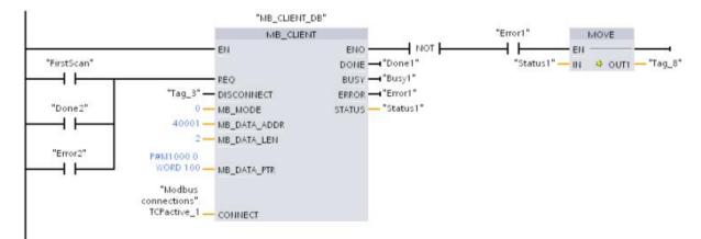
Network 1: Modbus function 3 - Read Modbus TCP server holding register words
