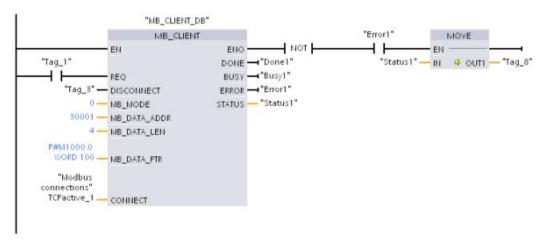
**Network 2:** Modbus function 3 - Read holding register words from a Modbus TCP server CONNECT parameter = "Modbus connections".TCPactive\_2: Connection **ID** = 2, **RemoteAddress** = 192.168.2.242, **RemotePort** = 502
