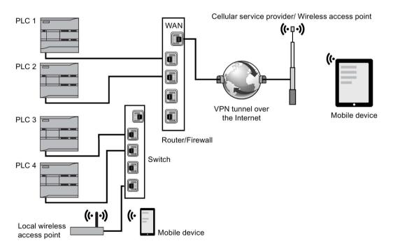
In this example, a mobile device that is within range of the local wireless access point can connect to PLC 3 and PLC 4 by their IP addresses. From the Internet outside the local wireless range, a mobile device can connect to PLC 1 and PLC 2 using the port forwarded address for each PLC.
