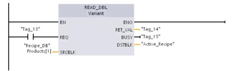
**Network 6** During run time, An HMI device could modify a component value stored in the Active\_Recipe DB. Improved recipe data can be stored by executing WRIT\_DBL. In the example, all Recipe\_DB start values for the single recipe "Recipe\_DB". Products[1] are overwritten by the current values from the "Active\_Recipe" DB.
