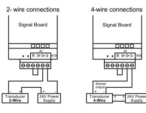
Table A- 205 Wiring diagram for the analog input SB
