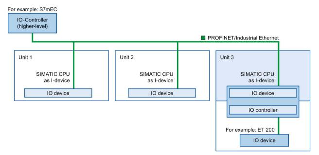
Unit 1 and unit 2 each consist of an I-device with centralized I/O. The I-device along with the distributed I/O system (for example, ET 200) forms unit 3.
