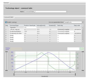
You can select the command types that are to be used for processing the command table. Up to 32 jobs can be entered. The commands are processed in sequence.
