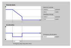
Dynamics: You can configure the motion dynamics and the behavior of the emergency stop command.
