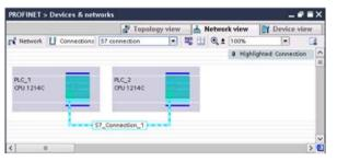
Click the "Highlighted: Connection" button to access the "Properties" configuration dialog of the communication instruction.
