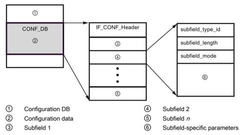
The configuration data of CONF\_DB consists of a field that contains a header (IF\_CONF\_Header) and several subfields. IF\_CONF\_Header provides the following elements:
