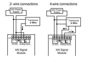
Table A- 151 Wiring diagrams for the analog input/output SM
