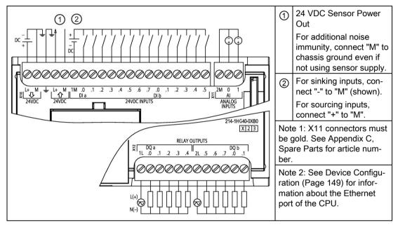
Table A- 61 Connector pin locations for CPU 1214C DC/DC/Relay (6ES7 214-1HG40-0XB0)
