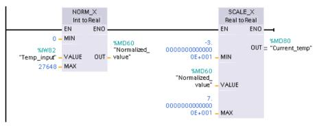
Note that if the analog input was from an analog signal module or signal board using voltage, the MIN value for the NORM\_X instruction would be -27648 instead of 0.
