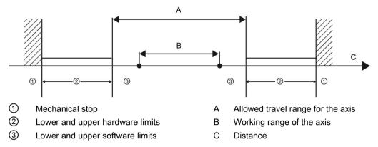
Hardware and software limit switches must be activated prior to use in the configuration or in the user program. Software limit switches are only active after homing the axis.
