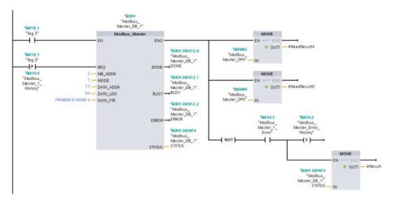
Network 4: Write 64 bits to the output image register starting at slave address Q2.0.
