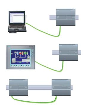
Programming device connected to the CPU
