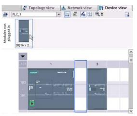
STEP 7 provides a storage area for "unplugged" modules. You can drag a module from the rack to save the configuration of that module. These unplugged modules are saved with your project, allowing you to reinsert the module in the future without having to reconfigure the parameters.
