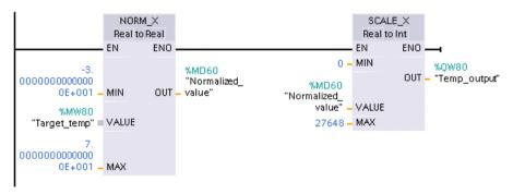
Note that if the analog output was for an analog signal module or signal board using voltage, the MIN value for the SCALE\_X instruction would be -27648 instead of 0.
