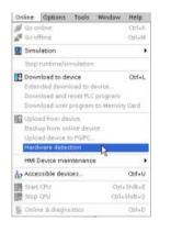
If you are connected to a CPU, you can upload the configuration of that CPU, including any modules, to your project. Simply create a new project and select the "unspecified CPU" instead of selecting a specific CPU. (You can also skip the device configuration entirely by selecting the "Create a PLC program" from the "First steps". STEP 7 then automatically creates an unspecified CPU.)
