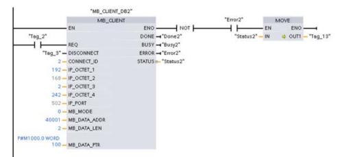
Network 2: Modbus function 3 - Read holding register words from a Modbus TCP server
