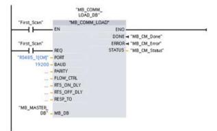
One MB\_MASTER instruction is used in the program cycle OB to communicate with a single slave. Additional MB\_MASTER instructions can be used in the program cycle OB to communicate with other slaves, or one MB\_MASTER FB could be re-used to communicate with additional slaves.
