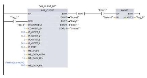
Network 1: Modbus function 1 - Read 16 output image bits
