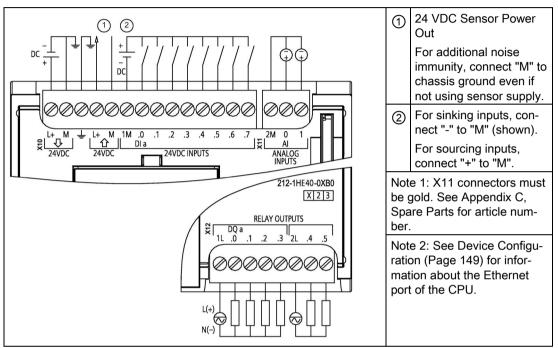
Table A- 43 Connector pin locations for CPU 1212C DC/DC/Relay (6ES7 212-1HE40-0XB0)
