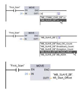
Entering a Modbus slave variable using the default DB name:
