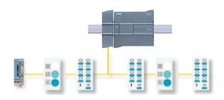
To use AS-i with S7-1200 V4.0 CPUs, you must upgrade the AS-i Master CM firmware to V1.1.
