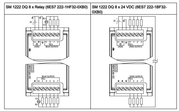
Table A- 112 Connector pin locations for SM 1222 DQ 8 x Relay (6ES7 222-1HF32-0XB0)
