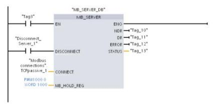
**Network 2:** Connection #2, Instance DB = "MB\_SERVER\_DB\_1, within "Modbus connections.TCPpassive\_2" (ID = 2 and LocalPort = 503)
