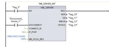
Network 2: Connection #2 with independent IP\_PORT, connection ID, and instance DB
