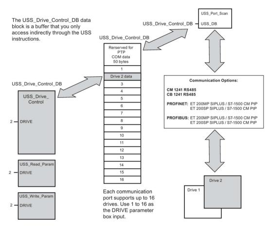
All drives (up to 16) connected to a single RS485 port are part of the same USS network. All drives connected to a different RS485 port are part of a different USS network. Each USS network is managed using a unique data block. All instructions associated with a single USS network must share this data block. This includes all USS\_Drive\_Control, USS\_Port\_Scan, USS\_Read\_Param, and USS\_Write\_Param instructions used to control all drives on a single USS network.
