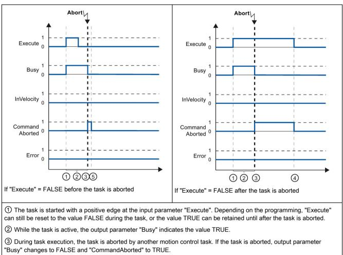
Table 10-87 Example 2 - If the task is aborted prior to reaching the parameterized velocity
