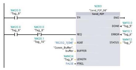
**Network 4:** monitor the DONE output of SEND\_PTP and reset the transmit flag (Tag\_8 at M20.0) when the transmit operation is complete. When the transmit flag is reset, the RCV\_PTP instruction in Network 1 is enabled to receive the next message.
