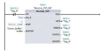
**Network 2:** Use the NDR value (Tag\_1 at M0.0) set by the RCV\_PTP instruction to make a copy of the number of bytes received and to set a flag (Tag\_8 at M20.0) to trigger the SEND\_PTP instruction.
