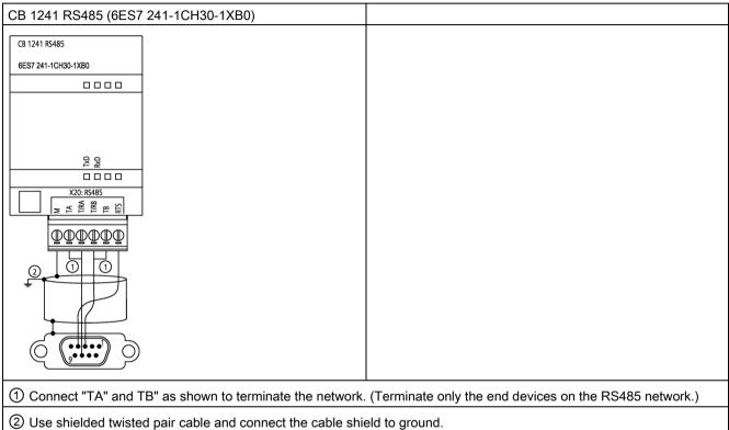
You terminate only the two ends of the RS485 network. The devices in between the two end devices are not terminated or biased. See the topic "Biasing and terminating an RS485 network connector" (Page 864)
