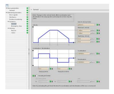
You can now change the value of any of your motion control configuration parameters as shown in the figure below.
