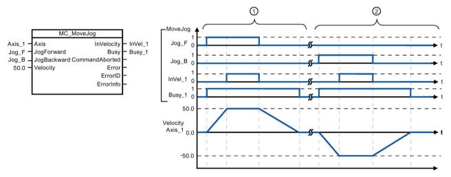
The following values were configured in the "Dynamics > General" configuration window: Acceleration = 10.0 and Deceleration = 5.0
