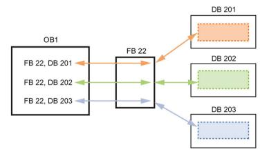
In this example, FB 22 controls three separate devices, with DB 201 storing the operational data for the first device, DB 202 storing the operational data for the second device, and DB 203 storing the operational data for the third device.
