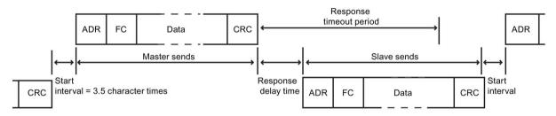
The response timeout period RESP\_TO is the amount of time a Modbus master waits for the start of a response from a Modbus slave. This time period is not defined by the Modbus protocol, but is a parameter of each Modbus master. The frequency of execution (the time between one execution and the next execution) of MB\_SLAVE must be based on the particular parameters of your Modbus master. At a minimum, you should execute MB\_SLAVE twice within the response timeout period of the Modbus master.
