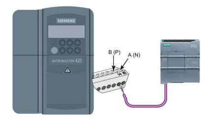
The terminal block connections are labeled numerically. Using a PROFIBUS connector on the S7-1200 side, connect the A terminal of the cable to the drive terminal 15 (for an MM420) or terminal 30 (MM440). Connect the B terminal of B (P) A (N) the cable connector to terminal 14 (MM420) or terminal 29 (MM440).
