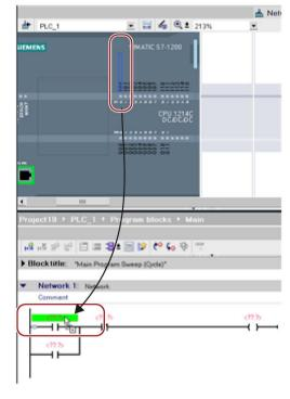
To help you perform tasks quickly and easily, STEP 7 allows you to drag and drop elements from one editor to another. For example, you can drag an input from the CPU to the address of an instruction in your user program.
