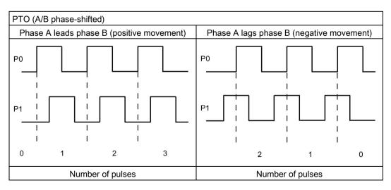
PTO (A/B phase-shifted - fourfold): If you select a PTO (A/B phase-shifted - fourfold) option, then both outputs pulse at the speed specified, but 90 degrees out-of-phase. The fourfold is a 4X configuration, meaning one pulse is the transition of each output (both positive and negative). In this case, the direction is determined by which output transitions high first. P0 leads P1 for the positive direction. P1 leads P0 for the negative direction.
